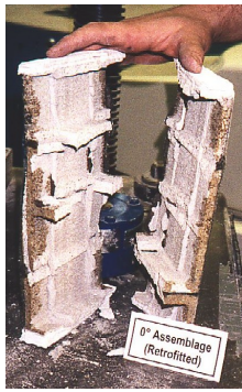
Figure 5: Failure mode of the retrofitted on/off-axis compression assemblages
