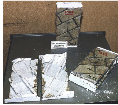
Figure 5: Failure mode of the retrofitted on/off-axis compression assemblages
