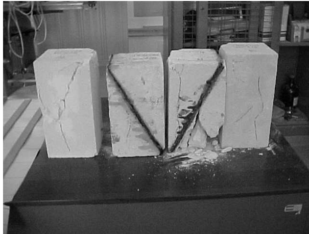
Figure 2 – Specimens for Bond Tests between CFRP Sheets and Masonry Blocks
