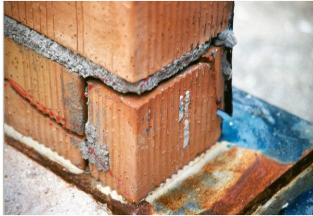
Figure 13 – View of local failure of the strengthened model
