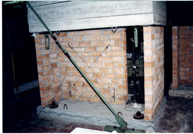
Figure 1 - Brickwork masonry model in scale 1 to 2.
