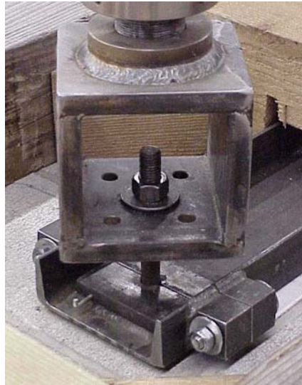
Figure 1: Details of the Attachment Between the Actuators and the Anchor Bolt
