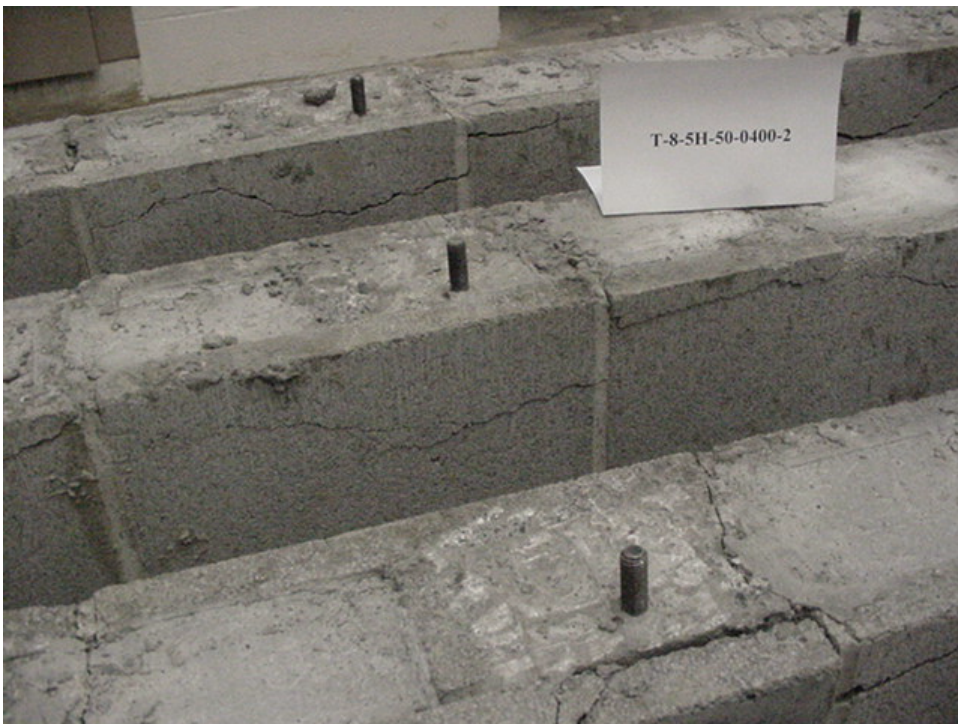
Figure 7. Failed Specimen T-8-5H-50-0400-2
