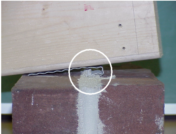
Figure 6. Compression Failure Mode: Buckling of Tie in Type NSCO Specimen
