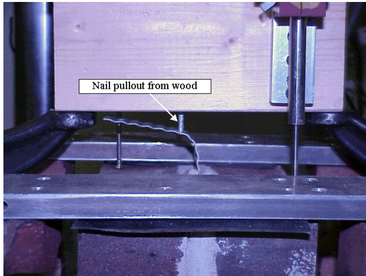
Figure 4. Tension Failure Mode: Nail Pullout from Wood in Type NSTE Specimen
