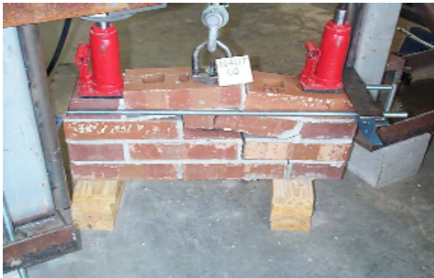
Figure 2- External Reinforcing Apparatus
