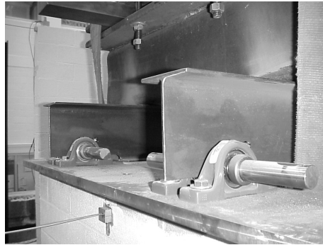
Figure 4. Diaphragm mass to out-of-plane wall connection detail.
