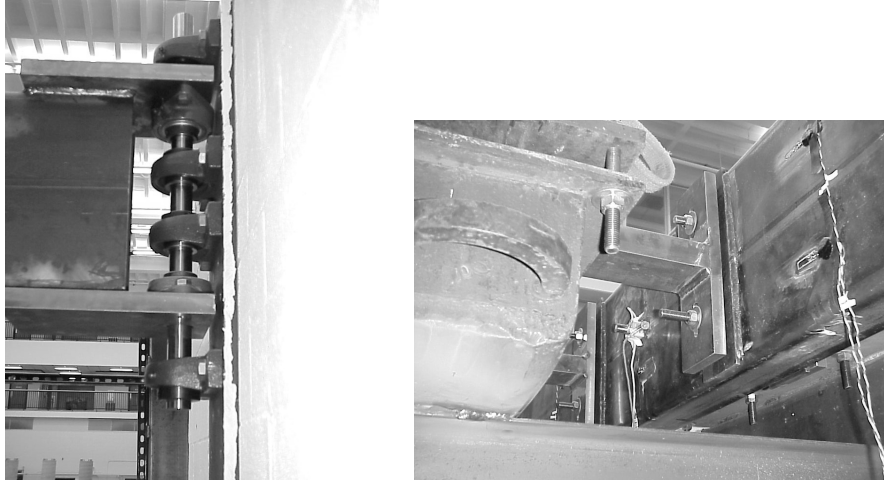
Figure 5. (a) Diaphragm beam to in-plane wall connection detail. (b) Diaphragm beam-to-diaphragm mass connection detail.
