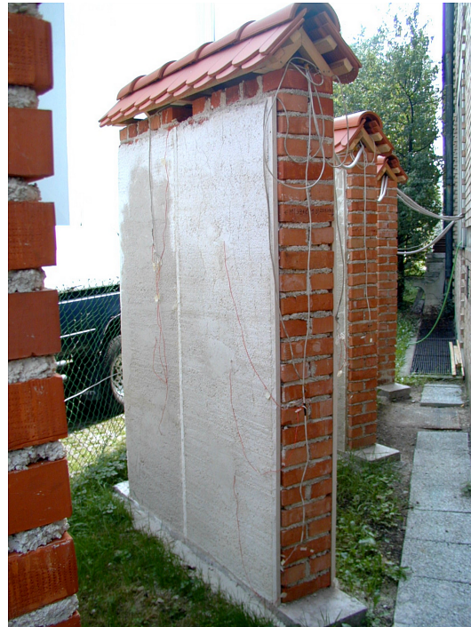
Figure 4. Rendered masonry walls
