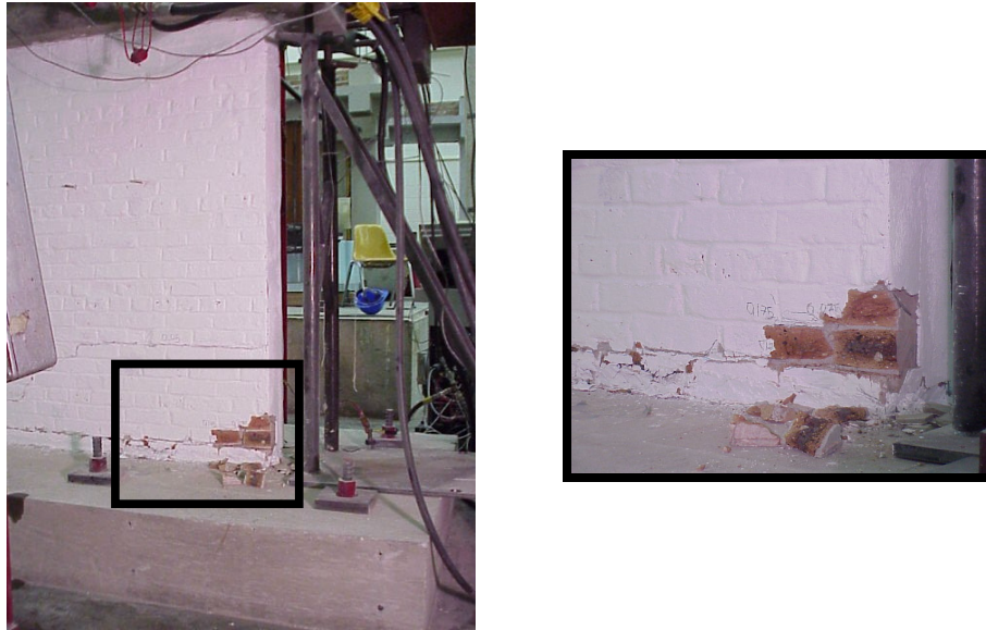
Figure 6 Toe-Crushing at the Ultimate Stage, Specimen 2S
