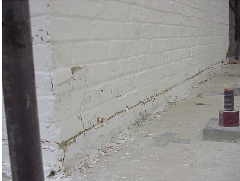
Figure 4 Sliding Along the Bottom Bed-Joint, Specimen 2S
