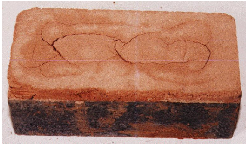
Figure 2. Shrinkage cracking of mortar within a flat bed using sand 438
