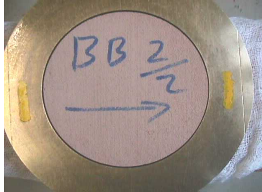
Figure 5: A view of the new test mould complete with specimen
