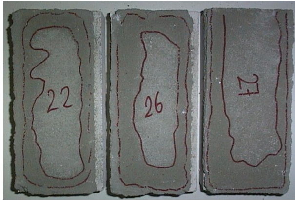
Figure 3. Examples of net bond area, 3 zones
