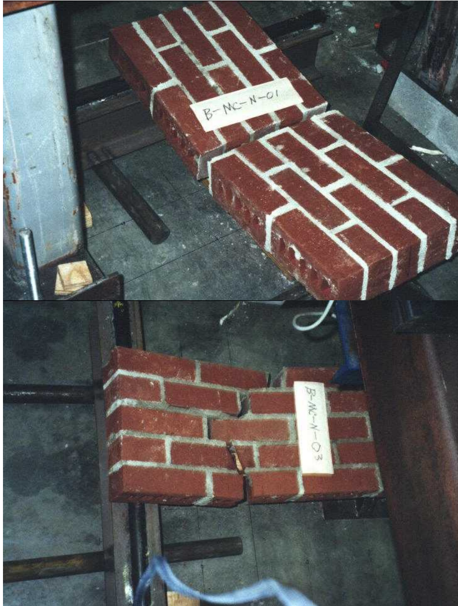
Fig. 7 - Failure Along a Zigzag Fracture Plane – Solid Brick Masonry Specimen
