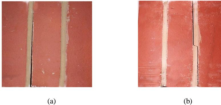
Figure 6 – Test specimens showing failure mode: (a) failure initiated by tensile stresses; (b) failure initiated by shear stresses
