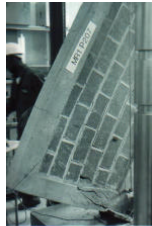
Figure 4 Typical Rotation of Brick Units for Rectangular Specimens
