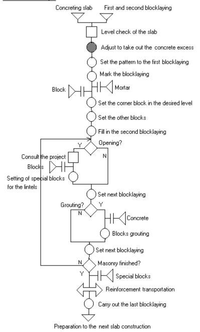
Figure 2: Flowchart of execution of the structural masonry.
