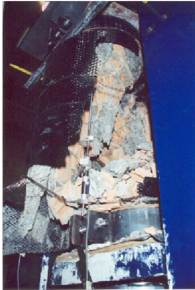
Figure 5. Circular section column after failure
