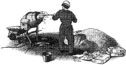
Fig. 8 Barrel type mortar mixer, (Illustration courtesy of Mega® Mix, Phoenix, AZ)
