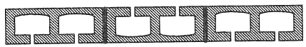
Fig. 13: Cross section through a wall constructed from resonant blocks facing in alternate directions.
