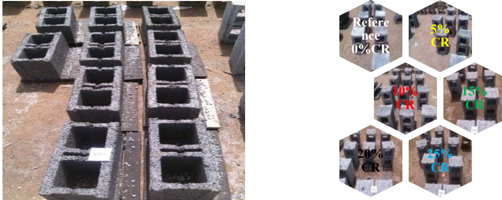
Figure 2: Manufactured Masonry Hollow Concrete Blocks
