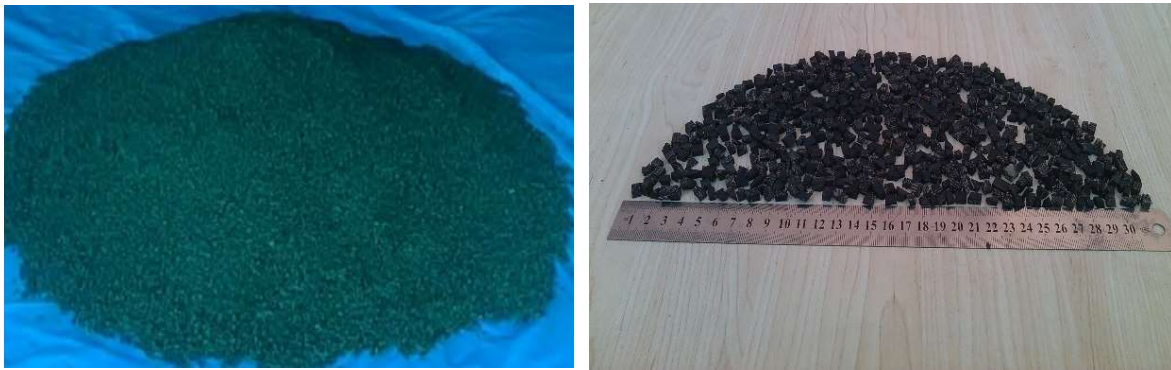
Figure 1: Crumb-Rubber Aggregate Used for Concrete Mix
