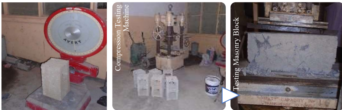
Figure 3: Weighing and Compressive Strength Testing of Masonry Hollow Concrete Blocks
