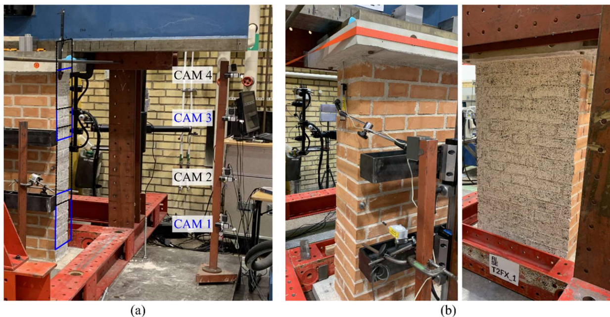
Figure 3: DIC Measurement Setup: 2D (a) and 3D (b)
