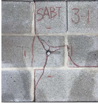
Figure 5: a) Radial cracks in SABT3-1 b) Break out cone with the anchor bolt undisturbed
