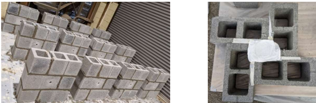
Figure 2: a) Anchor bolt test wall panels b) Formwork for compression test specimen
