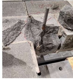
Figure 5: a) Radial cracks in SABT3-1 b) Break out cone with the anchor bolt undisturbed
