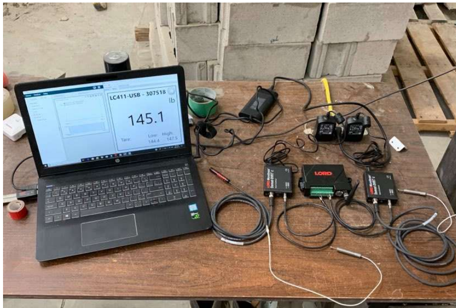
Figure 3: Displacement sensor and data acquisition set-up.
