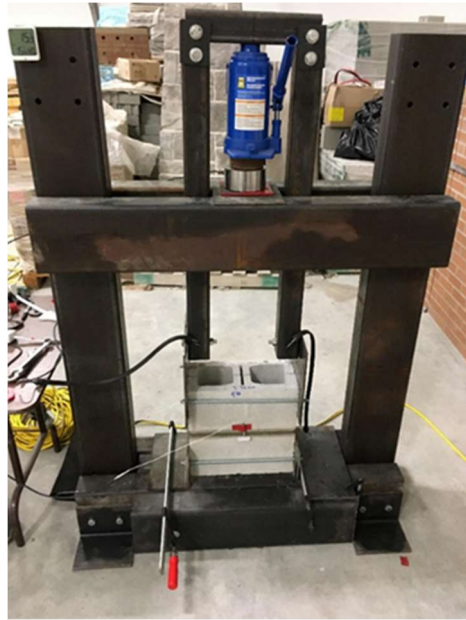
Figure 1: Testing apparatus configuration for tensile testing at CMDC.
