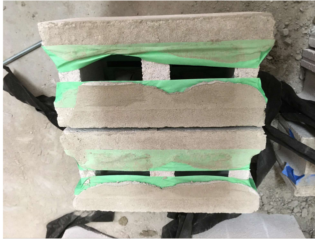
Figure 4: Typical failure pattern of early-age masonry assemblages under tensile loads
