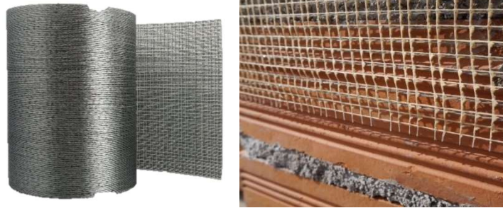
Figure 3: Steel Reinforced Grout (SRG)
