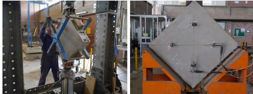
Figure 7: Test setup of the diagonal compression tests
