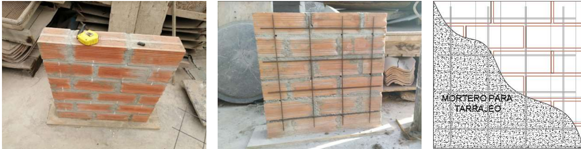
Figure 5. Wall specimen strengthened with welded wire mesh
