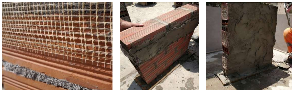
Figure 6: Small wall specimen reinforced with SRG
