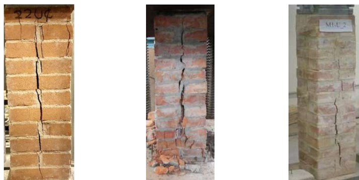
Figure 1: Brittle Failure of Unconfined Column [24-26]
