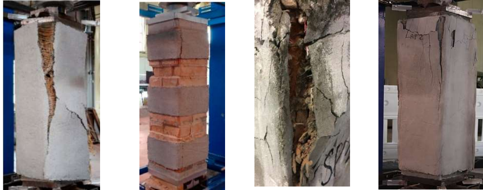
Figure 2: Failure configurations of confined columns [12,21,28]
