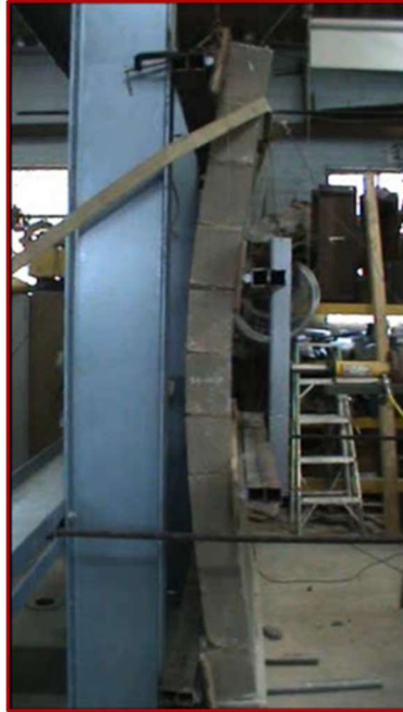
Figure 3: Concrete Masonry Test Panel with 4 – No. 4 GFRP Bars [6]
