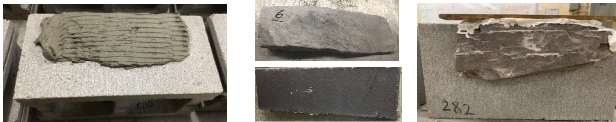
a) Conc block with mortar spread b) Thin stone/brick c) Specimen ready for testing
