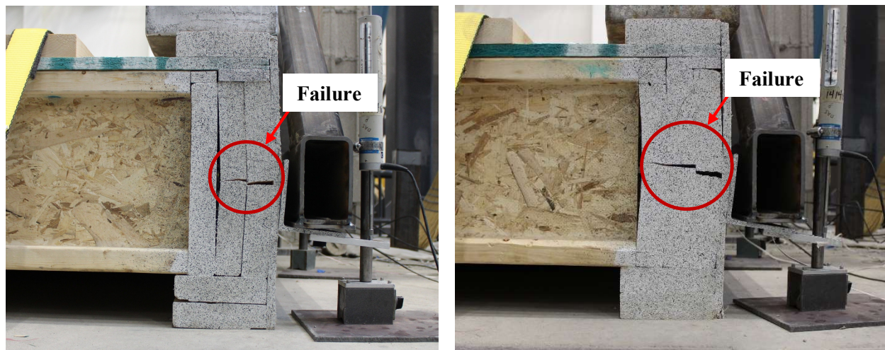
Figure 7: Splitting failure of the specimens built using (a) lag screws and (b) through-bolts
