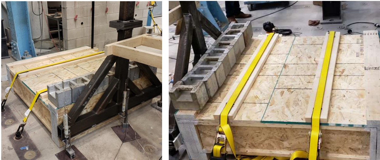
Figure 3: (a) Application of axial and gravity loads, (b) Straps used for anchoring the specimen
