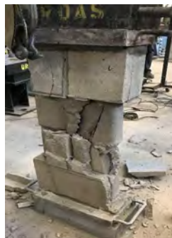
(a): Loading applied normal to bed joint
