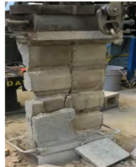
(b): Loading applied parallel to bed joint
