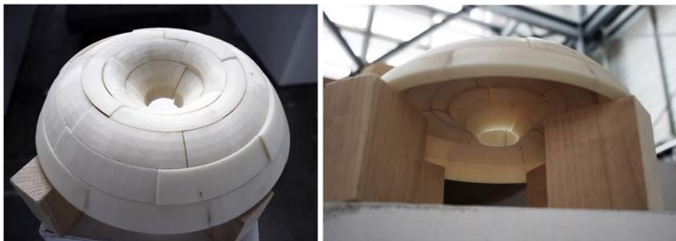
Figure 1: Ambidome exterior and interior: 3d printed ABS blocks, 240mm diameter
