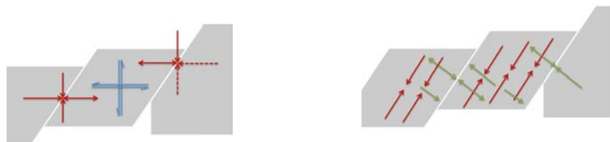
Figure 13: (Blue) Shear Action in Floor Dome and Arch; Resolved into Diagonal Forces
