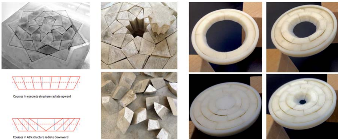
Figure 9: Conventional and Inverted Tapering of Voussoirs
