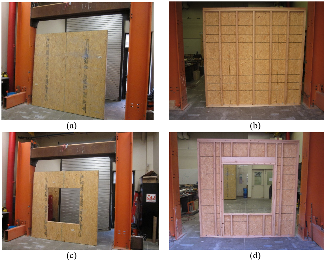
Figure 8: TWF 2.43m x 2.43m (8 ft x 8 ft) wall specimens: (a) front view with no opening, (b) back view with no opening, (c) front view with opening, (d) back view with opening
