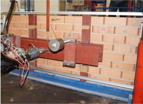
**Figure 9: Test set-up with built-in wall under four-point bending**
