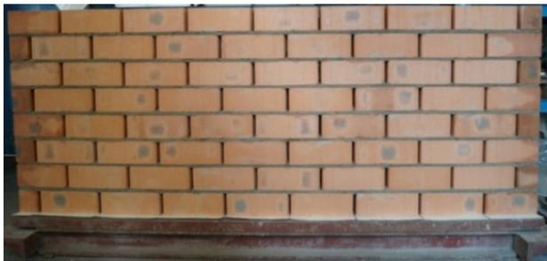
**Figure 7: Unreinforced masonry wall specimens**
