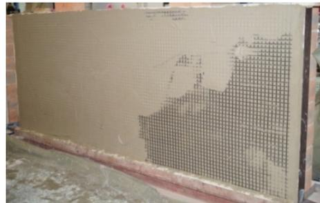
**Figure 8: Textile reinforced rendering applied on one masonry wall side**
