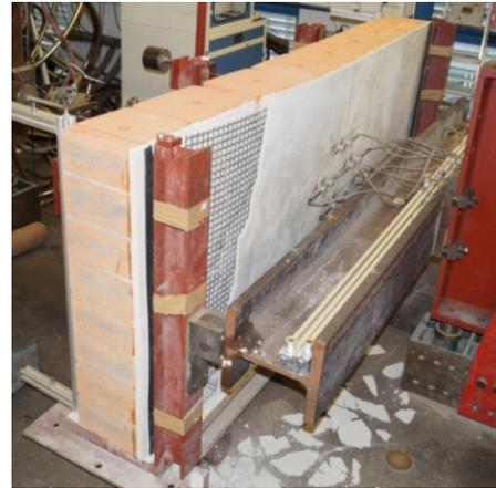
**Figure 12: Bond failure between render and textile of the reinforced wall w5**
