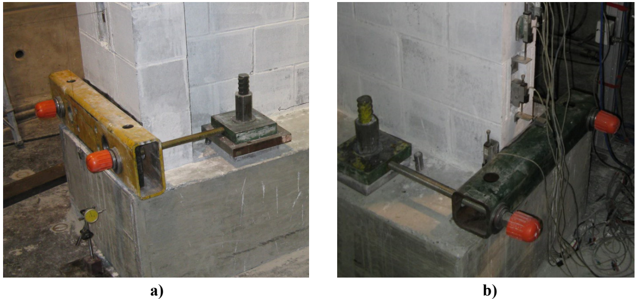
Figure 3: Sliding restraints at a flanged end-zone a), and at a web end-zone b).
