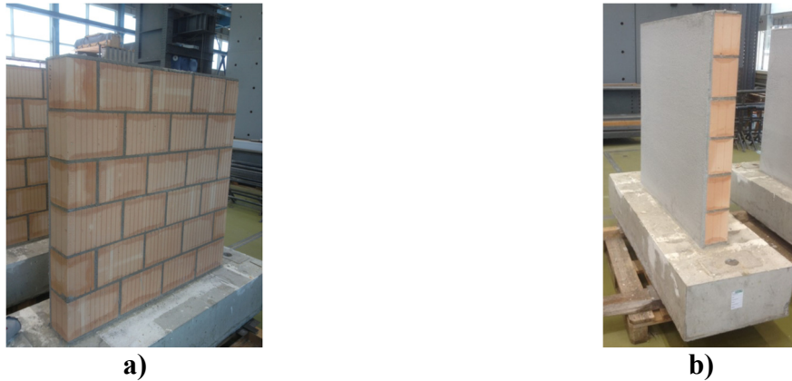
Figure 5: URM wall specimen: a) without plaster; b) with plaster
