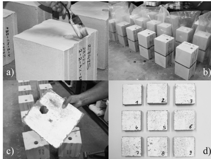
Figure 4: Manufacturing of 2-unit specimens and extraction of prisms
