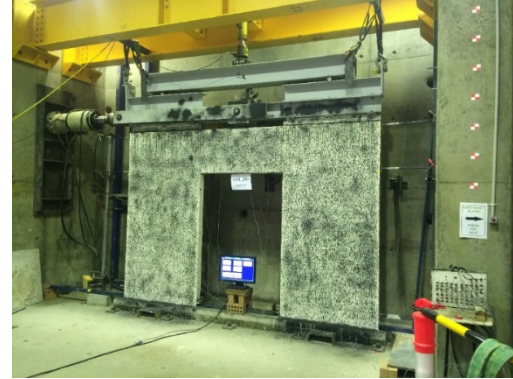
b) As-built test setup for wall W01_10a
