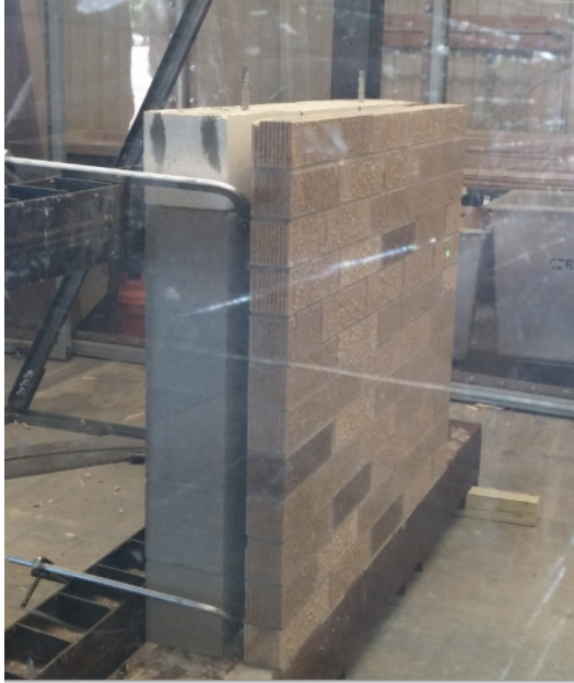
Figure 5: Utility Brick Unit Specimen 1 in Testing Apparatus Prior to Testing
