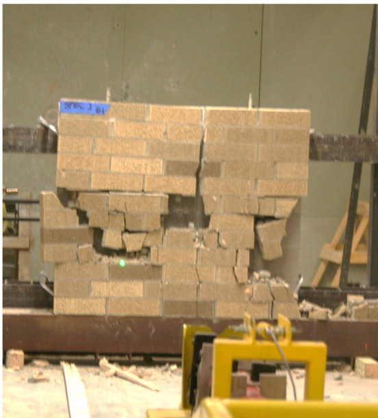
Figure 7: Veneer Damage on the Utility Unit Specimen 1 after Three Missile Strikes
