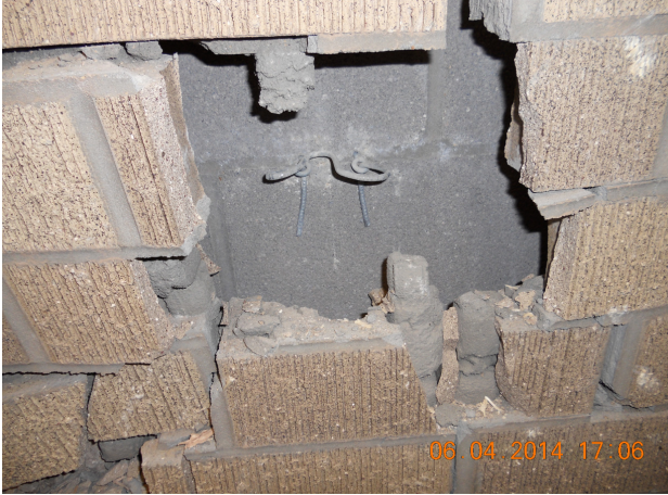
Figure 9: CMU Surface Behind Missile Strike on the Utility Unit Specimen 1 After Testing
