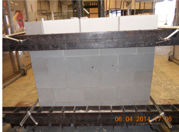
Figure 10: Back Surface of CMU on the Utility Unit Specimen 1 After all Three Missile Strikes
