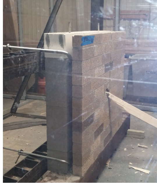
Figure 6: First Missile Strike on the Utility Unit Specimen
