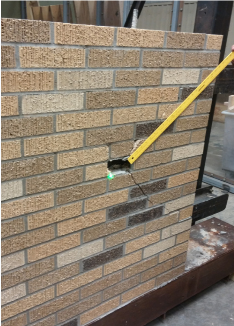
Figure 11: First Missile Strike on Modular Clay Veneer Specimen 2
