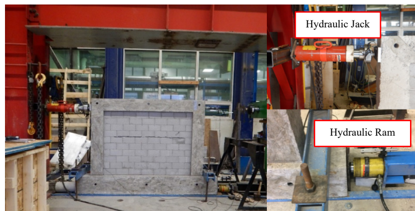
Figure 2: In-plane Test Setup
