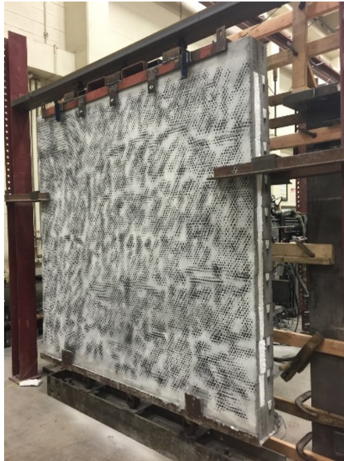
Figure 4: Out-of-Plane Flexure Test Frame
