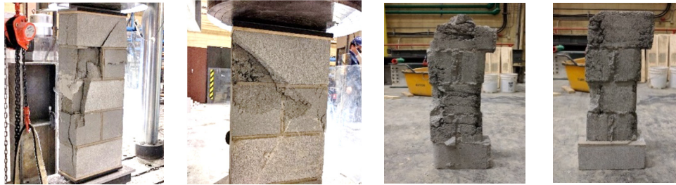
Figure 7: Failure modes ( e = t/6 )
