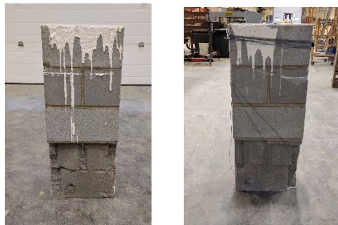
Figure 9: Eccentric Prism Failure ( e = 5t/12 )
