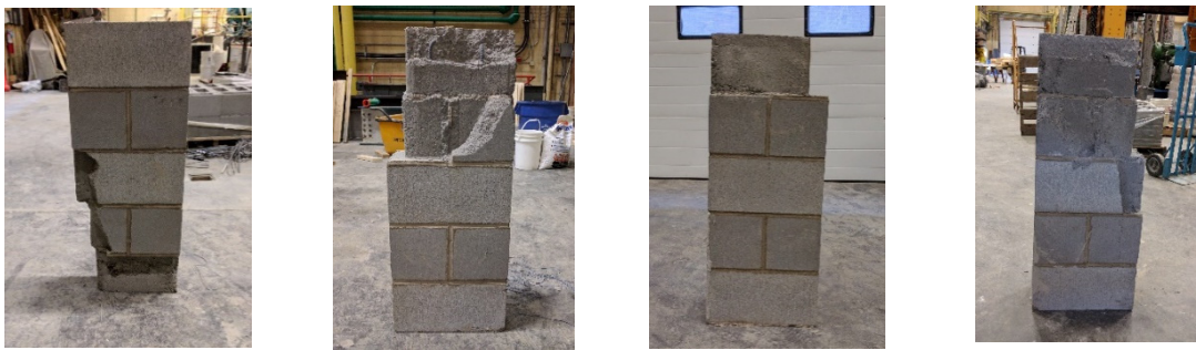
Figure 8: Eccentric Prism Failure ( e = t/3 )
