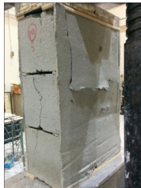
Figure 5: Concrete masonry prism strengthened by EDCC layers (5mm thick)
