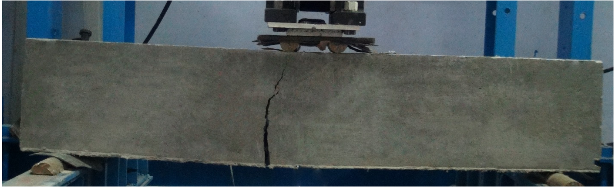
Figure 6: Failure mode of reinforced masonry beam with pultruded CFRP bars (Series #2)
