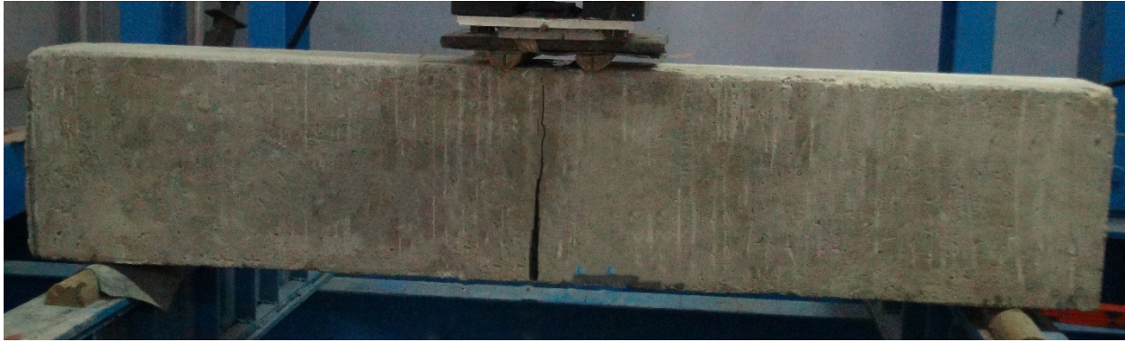
Figure 8: Failure mode of reinforced masonry beam with hand layup CFRP bars (Series #3)
