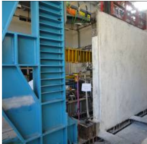
Figure 11: The Retrofitted Wall with Shotcrete Layer
