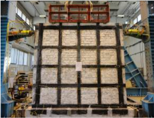
Figure 8: Configuration of CFRP Reinforcement
