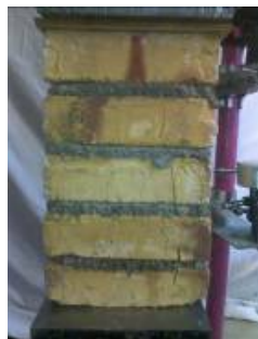
Figure 3: Cracking and Failure Pattern of the Specimen in Compression Strength Test
