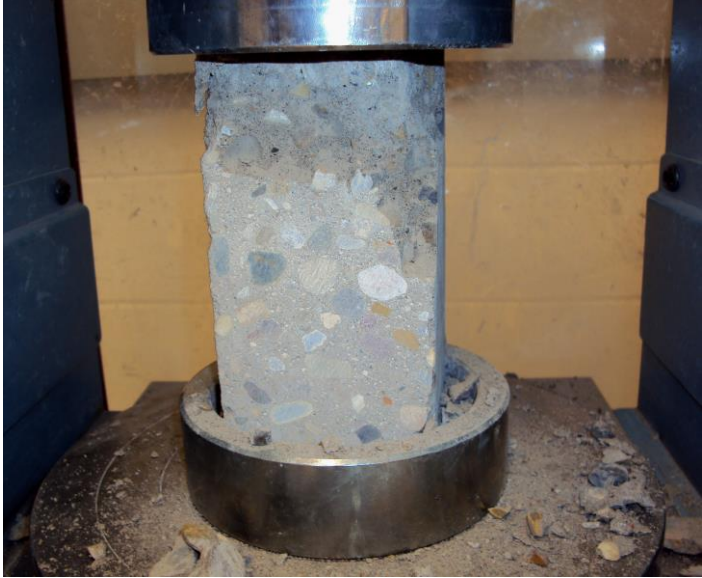
Figure 1: Test set-up for a Typical Prismatic Grout Core
