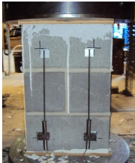
Figure 1: Set-up for Testing Grouted Masonry Prisms
