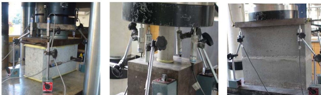
Figure 2: Axial compression tests a) Block; b) Mortar specimen; c) Prism
