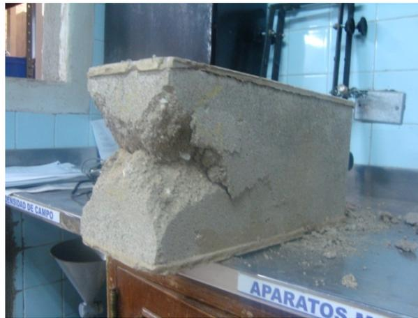
Figure 7. Failure diagonal cutting blocks typical of low and medium resistance.
