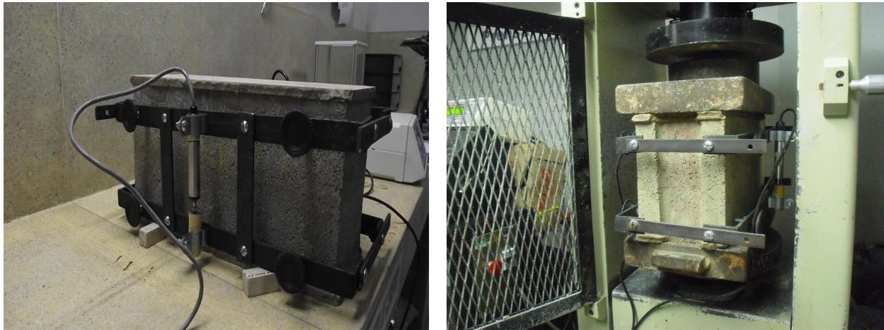
a) Concrete block test set-up
