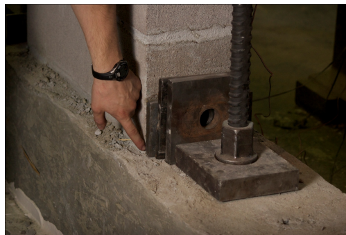
Figure 4: Plates to prevent sliding at base
