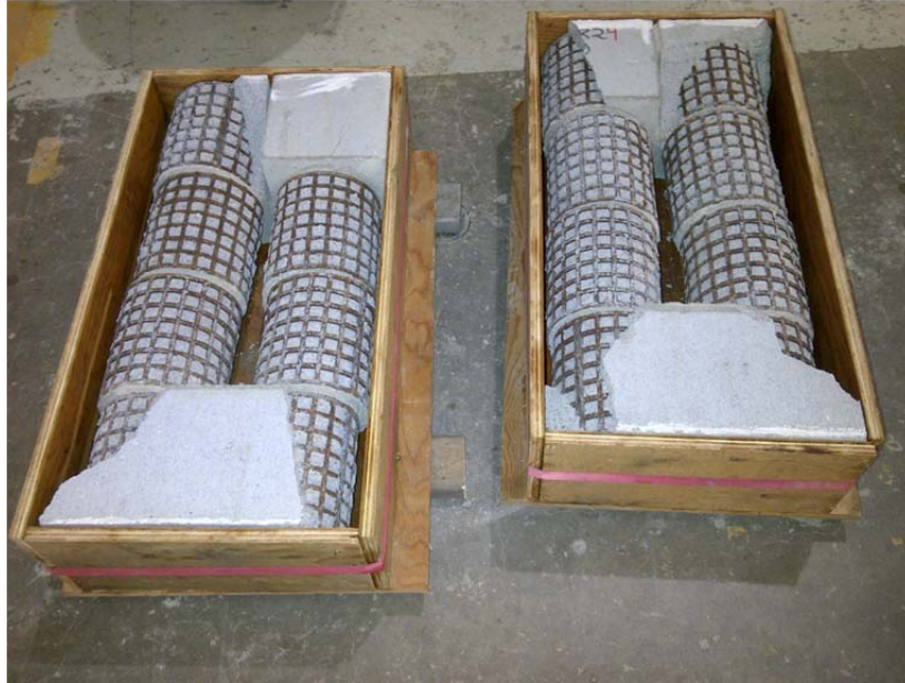
(a) Tested SR Block Prisms Positioned in Forms in Preparation for Repair
