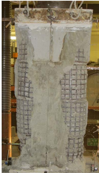
Figure 4: Repaired Prism #2 at Midtest
