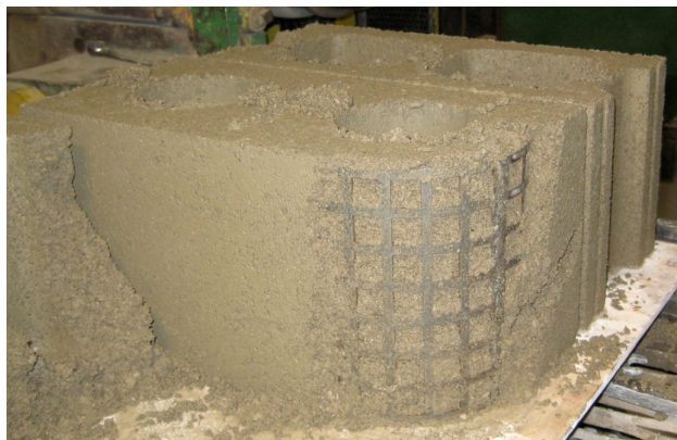
Figure 2: SR Block During Manufacturing with Confining Device Exposed by Removal of Compacted Exterior Concrete
